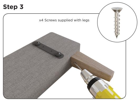
Use the supplied screw to secure the leg in place, stopping it from rotating out of position ( This step doesn't apply to cylindrical legs)
