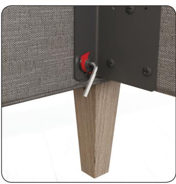
Use the allen key provided (A) to tighten the bolts onto the brackets
